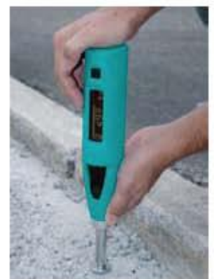
... on soft concrete (with mushroom plunger)
