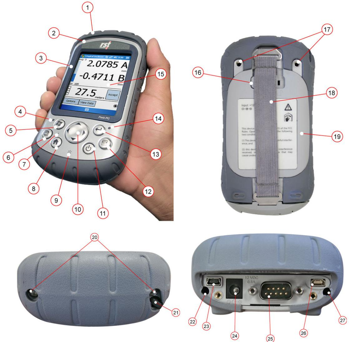
**Figure 8 – Overview of Ultra-Rugged Field PC**
