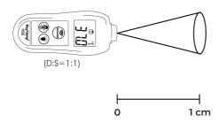
**EMISSIVITY** - The RayTemp HSE IR is supplied with a fixed default emissivity of 0.95. For information relating to the emissivity of specific materials, please visit our website etiltd.com/ emissivity. **Please note:** Non-contact infrared thermometers are not recommended for use in measuring the temperature of shiny or polished metals.
