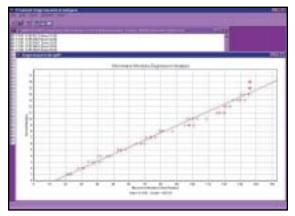
Computer display of the Trident's actual readings of moisture content within a sand test sample.
