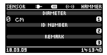
In this menu you can enter the diameter, the ID number of a measurement as well as a remark. Refer to the corresponding chapter for detailed information about these functions.
