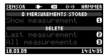
This menu shows the number of stored measurements. You can show stored measurements and also the last measurement or all measurements can be deleted. Refer to the corresponding chapter for detailed information about these functions.
