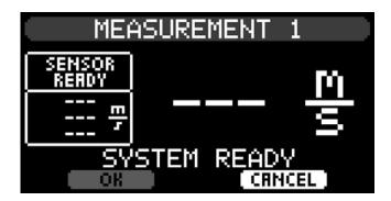
On the left side the sensor status will be displayed as well as the last 3 measurement values received by the sensor. On the right side appears the output of the actual measurement value. Right above the buttons the status of the system is displayed.
