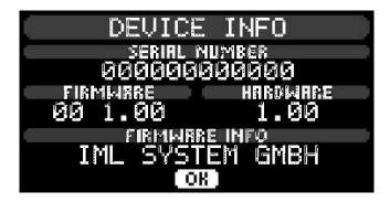
There are displayed the serial number of the electronic unit, the firmware version and the hardware revision.
