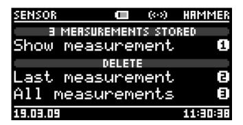
To show a saved measurement, press key 1. Page 1 of the last measurement is displayed:
