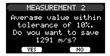
Choose **YES** to save the measurement and quit. Choose **NO** to not save it and to continue with the measurement. After saving the measurement, the measurement will be displayed. For more details read chapter *Showing a Measurement* in this manual. It is also possible to disable the automatic display of a measurement. For more details read chapter *System control, General information*.
