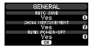
With **AUTO SAVE** you can determine whether it is suggested to save the measurement automatically if the last 3 measurement values were within a tolerance of 10 %.
