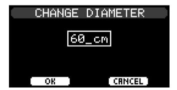
By the help of keys **0** to **9** you can enter the new diameter. Press the key below to delete the last char:
