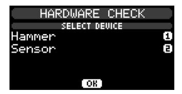
Select the option **Hammer** to check the hammer. A dialogue will appear, displaying the status of the hammer. Hit the impact cap to check if the hammer generates a correct signal:
