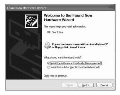
Mark the first option and select **Next**. The hardware wizard will install the new hardware. After the successful installation your PC can transmit data via USB and you can use M-Tools Light.
