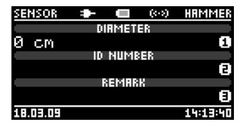
Press again the button on the left side to switch off the electronic unit. Keep pressed until the electronic switches off. Only if the main menu A, the main menu B or the system control menu is displayed the electronic unit can be shut down (see next paragraph).
