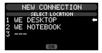
Select the storage location where the new connection has to be stored. There can be stored at most 3 connections. If you select a storage location that is already used by another connection, this connection will be overwritten by the new connection.
