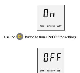
If the unit detects no key press for 2 seconds in the Setting screen, it moves to the next setting.
