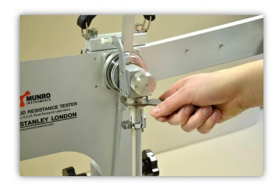
1.3 Position the instrument on the test surface. Use the spirit level and the three levelling screws to set the tester. Knurled spring-loaded locking nuts are provided to allow adjustment of the levelling screw tension.
