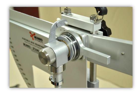
2.4 With the pendulum arm free and hanging vertical, place the setting spacer under the slider lifting handle setting screw to raise the rubber slider. The spacer can be found attached by a chain to the rear leg. Unclamp the locking knob and lower the head unit using the vertical movement control knobs until the rubber slider just touches the test surface. Clamp the head unit in position using the locking knob. Remove the spacer. The *approximate* sliding length has now been set.
