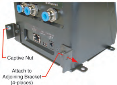
Fig. A-4 Attach Adjoining Bump / Cal Stations
