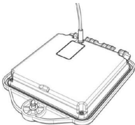
Figure 4.13 Charging the transmitter Li-ion battery pack
