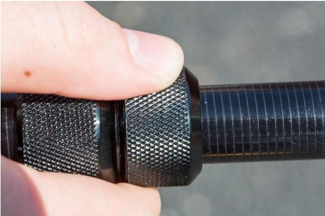
Fig. 6: Loosen Lower Pole section first, and pull out.
