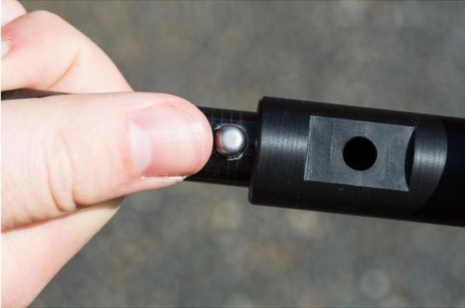
Fig. 7: Attach the Extension Pole to Sensor Adaptor piece. Snap in place.
