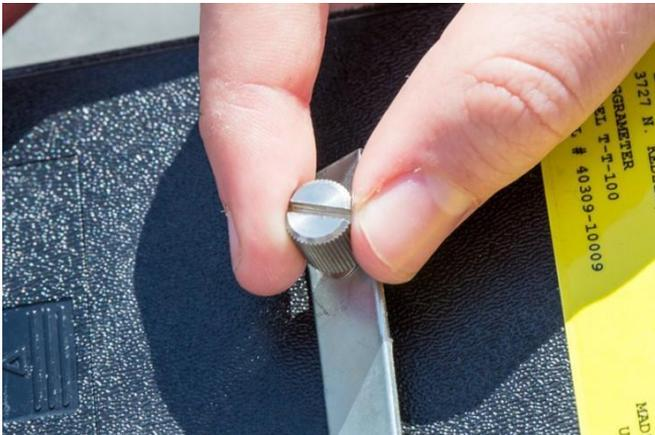
Fig. 8: Attach Bracket to bottom of Aggrameter® test unit.
