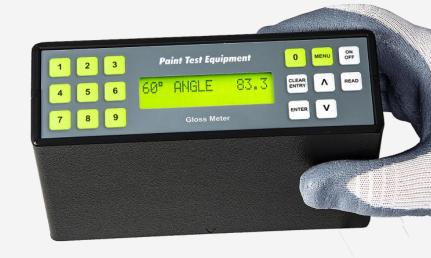
Gloss is measured with angles of 60° and 20°. The 60° angle is universal for all applications. The 20° angle gives improved differentiation of measurement on high-gloss coatings above 70 gloss units.
