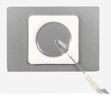
Completely fill the Syringe with the Deionised Water from the Beaker, and then empty the Syringe back into the Beaker.
