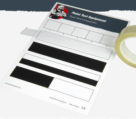
Remove a piece of Tape about 250mm long. Holding the Tape only at the ends, press approximately 200mm of the freshly exposed Tape onto the blast-cleaned surface.
