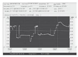
The field above the graphic display contains information on the time, sampling rate, number of data, alarm settings and the maximum, minimum and average values).
