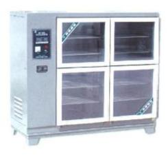
The box can carry out standard curing for concrete sample. Stainless steel plate from developed countries is use for the internal bladder. The spray employs ultrasonic humidification, high-power compressor, double-layer vacuum glass door and intellectual instrument with digital display of temperature and humidity, equipped with micro-printer, which is an idea unit for curing of concrete samples in testing laboratory and quality inspection center
