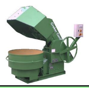
The advanced design of the **Croker Rotating Pan Mixer** range incorporates twin drives with separate geared motor units powering the rotating pan and mixing star, which together with the twin spring mounted mixing blades and fixed scraper blade enables the mixers to produce the high quality mix for which they are renowned.
