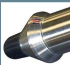
Close up of tip showing top (centre) reference markings which are used for proper orientation during operation.
