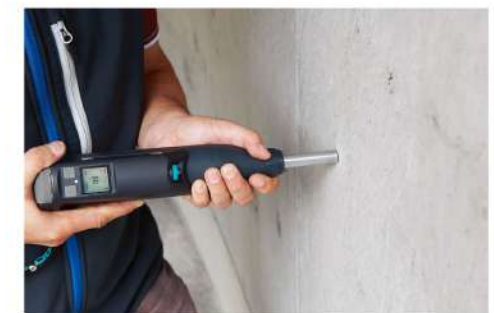
Original Schmidt Live with digital display
