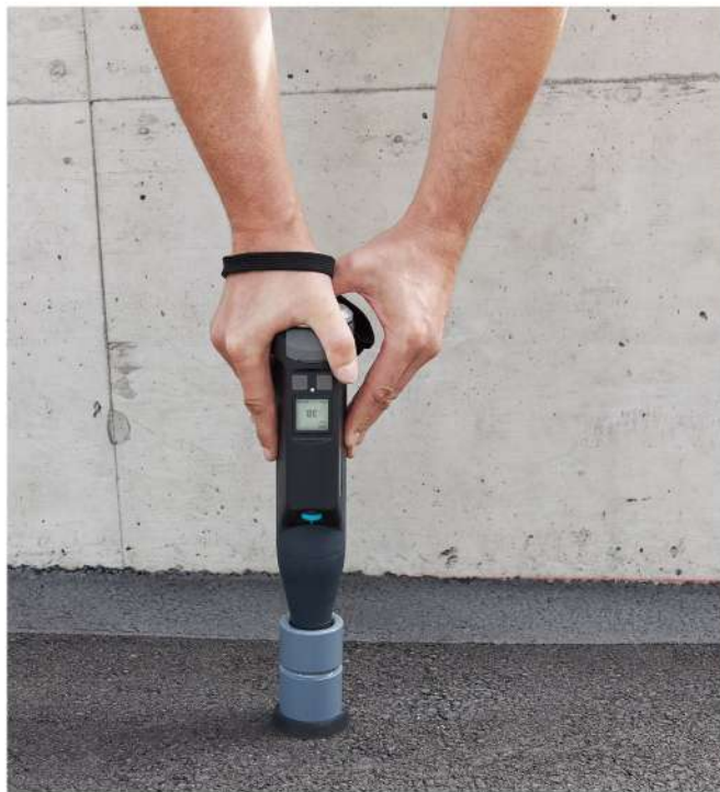
Original Schmidt Live with portable testing anvil
