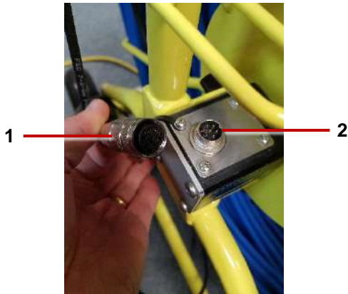
Fig. 4.2: Link cable (1) connects to the pushrod reel (2)
