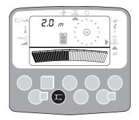
Press the Depth key to calibrate. The Receiver will display the calculated depth, beep twice and return to the DataSonde mode.
