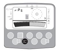
If during calibration the LCD displays 'rpt', repeat the calibration procedure checking that the Receiver to bore head distance is within 1.5 - 2.5 m (5 - 8 ft) parameter.
