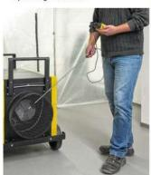
The slim telescopic probe of the TA300 can be variably extended to an effective length of 1 m, thus measuring applications can be carried out with more ease. Also convenient for flow rate measurements in remote or poorly accessible locations or inside air ducts and ventilation shafts.
