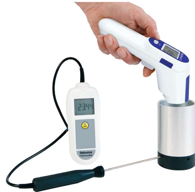
A Comparator being used to check the temperature of a RayTemp 3 Infrared thermometer against a Reference thermometer.
