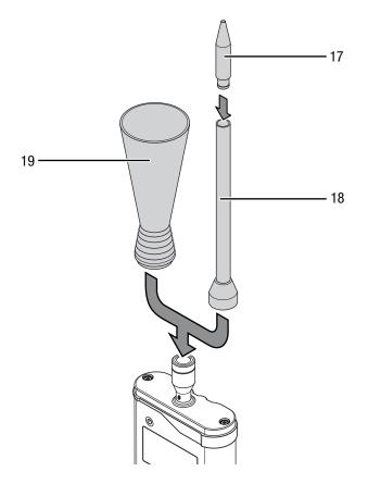
2. If you no longer need the adapter, carefully pull it off the airborne sound probe.
