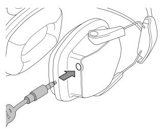
Plug the other jack plug into the device's headphone 2. connection.
