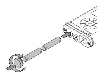
3. Screw the cover back onto the battery compartment.
