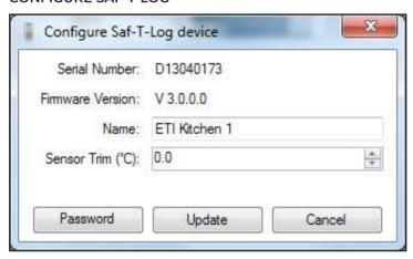
Click 'Configure Saf-T-Log' to assign a name or ID tag to a Saf-T-Log thermometer or adjust ('Sensor Trim') the Saf-T-Log. The serial number of the Saf-T-Log thermometer that is connected is displayed at the top of this window. Once the desired settings are completed, click 'Update' to immediately update the connected Saf-T-Log thermometer.
