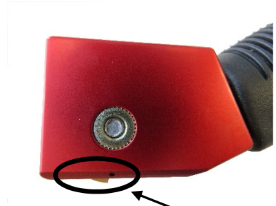
Correct inserting of the cutting tool
