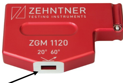
ZGM 1120 with adjusted measuring distance without the ACC742 mounting device
