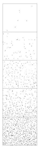
**1.** Particles not visible under X10 magnification.
