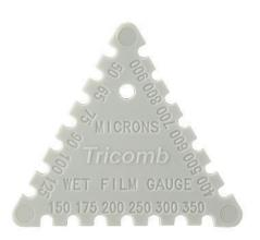
The Tricomb Plastic Wet Film Gauge ensures the quality control of the paint thickness while the coating is still wet. Applying too much coating can be expensive. Wet film measurements are also useful for coatings where the dry film thickness can only be measured destructively.
