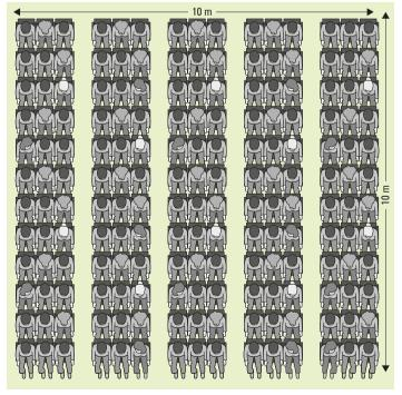
**Example of occupancy in large-capacity jet:** airlines are allowed to place the equivalent of 196 passengers on the same area – 0.51 m² room area per passenger – although only 19.3 m³ of clean air per hour are generated for each passenger – almost 8 times less than in the example call centre!
