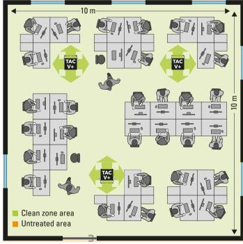
**Example of occupancy in a call center:** With an area of 10 x 10 m at a room height of 2.5 m, the office zone shown has an air volume of 250 m³, which 3 TAC V+ can circulate 19 times per hour (air capacity 4,800 m³/h), which corresponds to an air exchange rate (LW/h) of 19 (clean air volume of 150 m³ per person with 32 occupied workplaces) — almost a factor of 8 compared to the aircraft!
