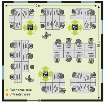
**Example call center:** With an area of 10 x 10 m at a room height of 2.5 m, the office zone shown has an air volume of 250 m³, which 3 TAC V+ can circulate 19 times per hour (air capacity 4,800 m³/h), which corresponds to an air exchange rate (LW/h) of 19.
