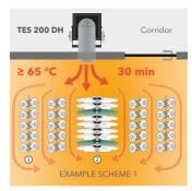
Application example 1: TES 200 DH placed outside the treatment room with piped air supply into the room. There the respiratory masks to be reprocessed are collected (1), for example on mobile shelf trolleys, and also contaminated tunics, gowns, trousers etc. on gown stands (2).
