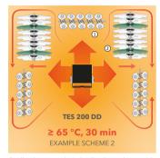
Application example 2: Application as in example 1, but with TES 200 DD placed directly in the decontamination room.
