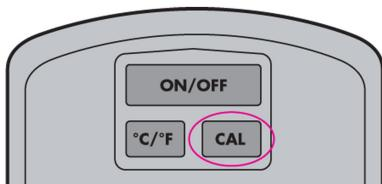
Press and HOLD DOWN the CAL button for a count of 5 seconds.
