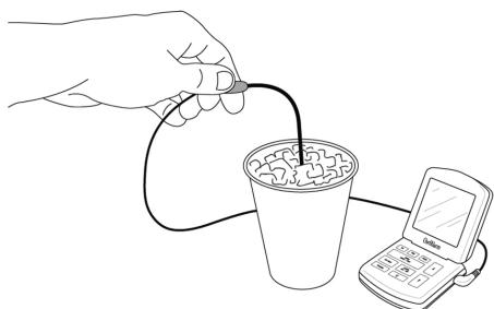
Repeat the ice bath test in Step 1. You should be spot-on or within  $\pm 0.05$  °C.
