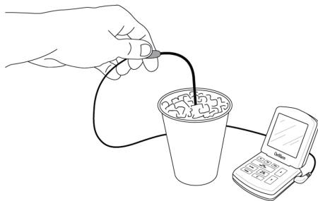
Turn the ChefAlarm on and immerse the probe into the ice bath and gently stir. When the temperature is stable and constant, note the final reading. It should be close to 0 °C. However, it may be low or high by several tenths of a degree or even one or two whole degrees. If, for example, the reading is -0.3 °C, then you are reading low by 0.3 °C.
