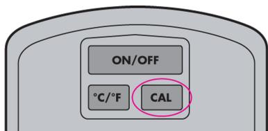
Press the CAL button one more time and the offset amount will be saved to the ChefAlarm. Now all readings will be 0.3 °C higher than before the CAL adjustment.
