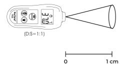
**EMISSIVITY** - The RayTemp HSE IR is supplied with a fixed default emissivity of 0.95. For information relating to the emissivity of specific materials, please visit our website etiltd.com/emissivity. **Please note:** Non-contact infrared thermometers are not recommended for use in measuring the temperature of shiny or polished metals.
