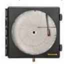
Pressure recording with a full 8-inch (203mm) diameter chart. These 8" (203mm) easy-to-ready pressure charts show 3x as much data as our 4" (101mm) and they are contained in a splashproof enclosure. Create a permanent visual record of your pressure data with the greatest detail.
