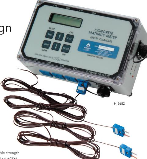
Humboldt Maturity Meters provide a predictable strength determination of cast-in-place concrete based on ASTM Standard C1074-98 (Estimating Concrete Strength by the Maturity Meter Method). These units utilize inexpensive, disposable, T-type thermocouple wire with quick-connect jacks, which can be embedded directly into a concrete structure to measure temperature at timed intervals. These readings can then be used to document the maturity process within the structure in order to:
